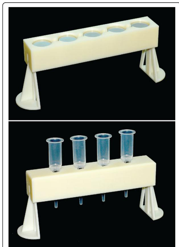
**Figure 3 Magnetic purification stand.** Photographs of the designed magnetic purification stand. (A) The stand with the lid removed showing the cylinder magnets. (B) The complete stand with four LS columns in place for purification. A disposable trough commonly used in high-throughput microplate applications fits beneath the column nozzles.
